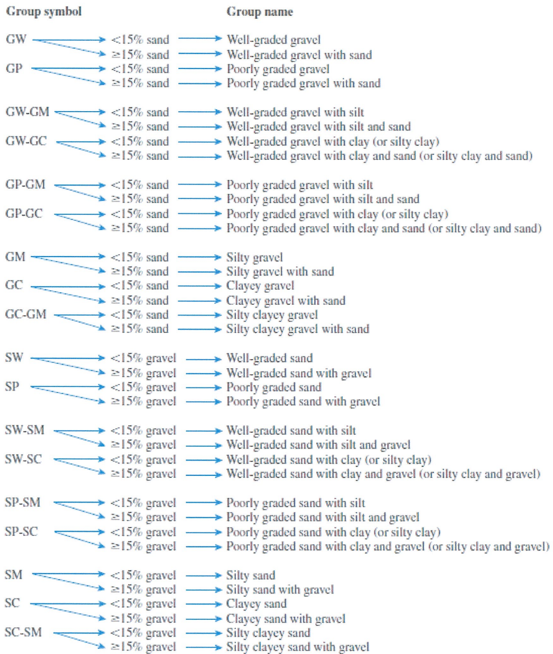
FIGURE Q1(b)(iii): Flowchart group names for gravelly and sandy soils
