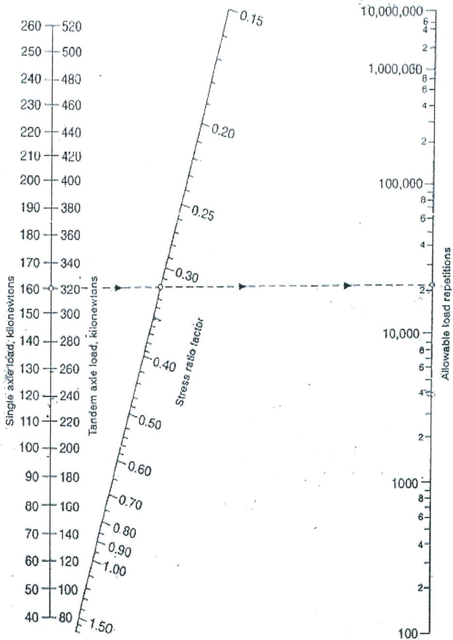
**FIGURE Q2 (c):** Fatigue analysis- Allowable load repetitions based on stress ratio factor (with and without concrete shoulder)
