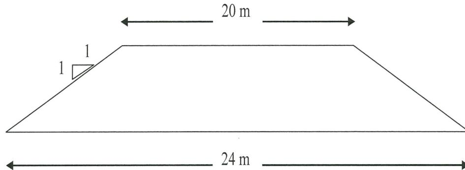
**Figure Q3:** Cross section of the embankment**Table 4:** Density and moisture content of the soil
