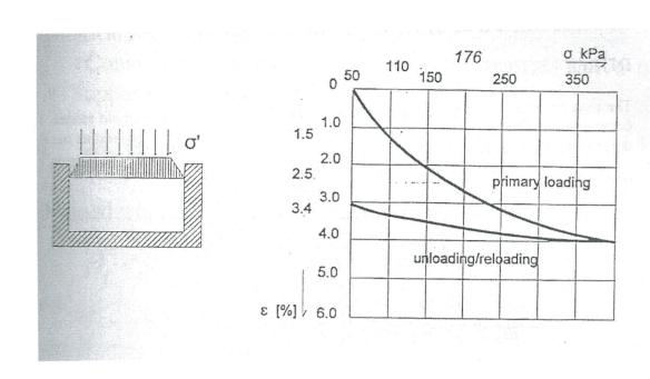
Figure Q3(e): Result from Oedometer
