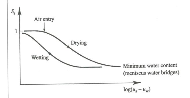
Figure Q1(d): SWCC of saturation vs soil suction
