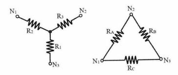
$$R_{1} = \frac{R_{B}R_{C}}{R_{A} + R_{B} + R_{C}} \qquad R_{A} = \frac{R_{1}R_{2} + R_{2}R_{3} + R_{3}R_{1}}{R_{1}}$$
