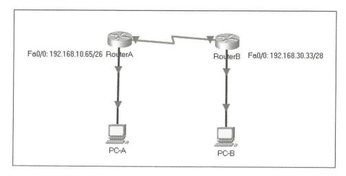
RouterA has an IP address of 192.168.10.65/26 and RouterB has an IP address of 192.168.30.33/28. The routers have been assigned with the first usable address.
