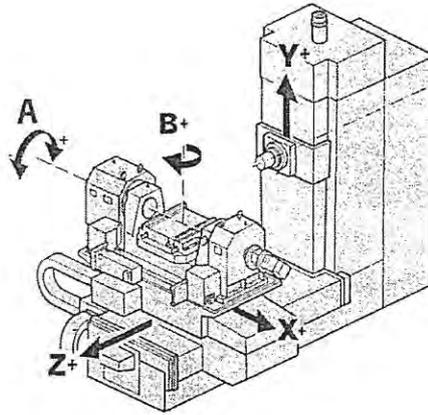
Figure Q2(a)(i): CNC Machine Configuration
