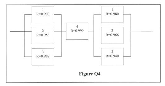
(e) Calculate the reliability of the system in **Figure Q4**.
